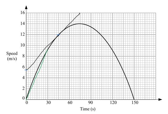
(a) Work out an estimate for the distance the car travelled in the first 30 seconds.
